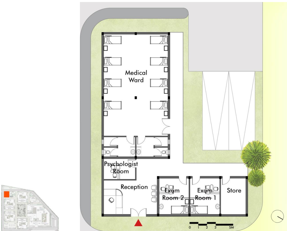
Figure 132. Plan of Infirmary
