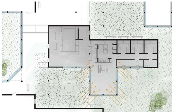
Figure 51. Use of Glass Brick Walls on Southern Facade to Allow Natural Light <Architizer>
