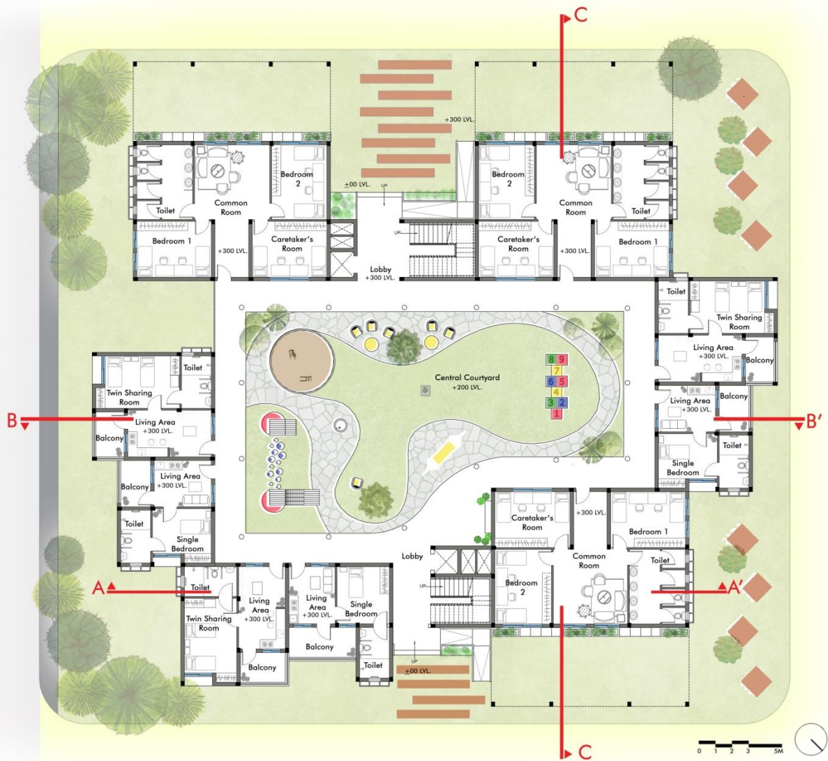
Figure 106. Cluster Plan - Ground Floor
