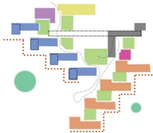
Figure 50. Staggered Arrangement of Units to Allow Sun <Author>
