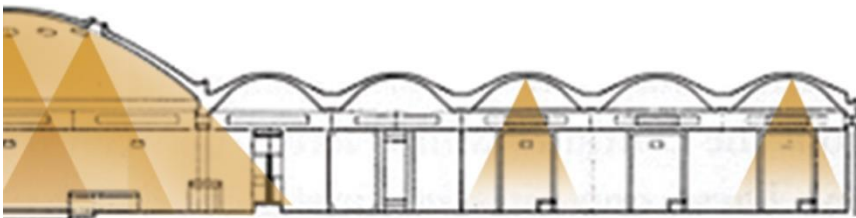
Figure 49. Section Depicting Light Entering Through Skylights
