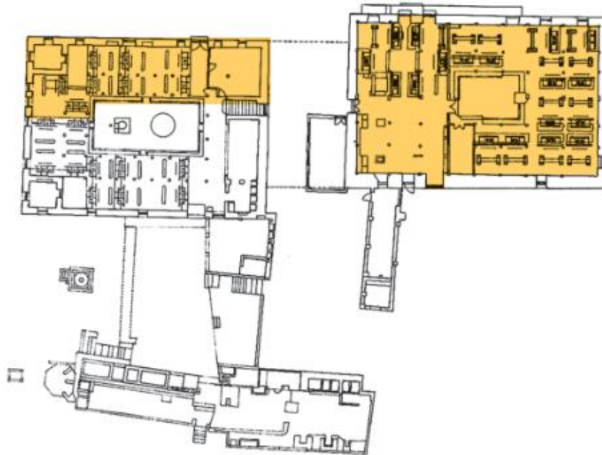
Figure 17. Present ground and first floor layout at the Rehwa Society. The Highlighted portions depicts the latest addition of the weaving spaces on the ground and first floor.
