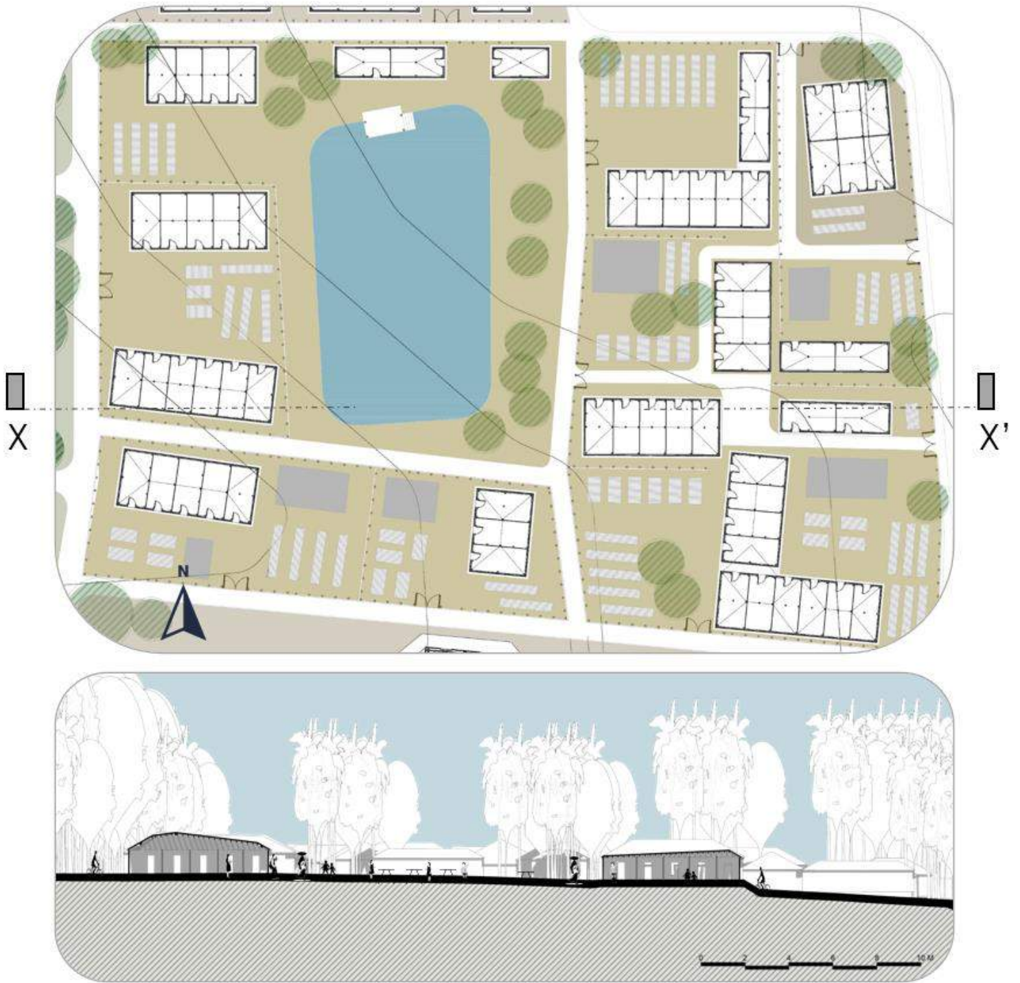
Figure 87 Cluster Plan and Section for Transient Fish Processors (Source: Author)
