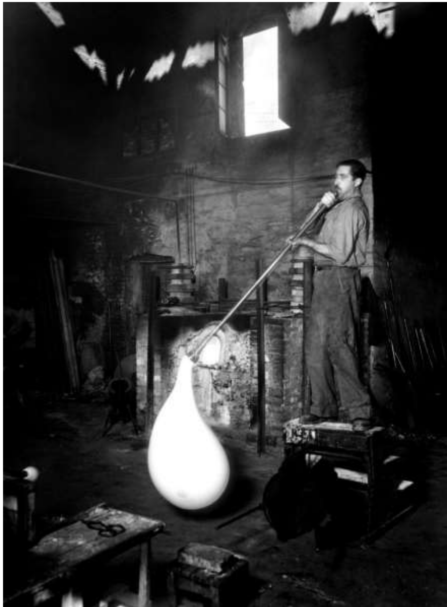
Figure 32: Making of Venetian glass
