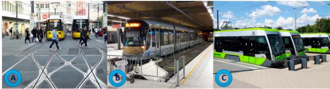
Figure 10: Tram route terminals without applying tram loops (A) Germany (B) Belgium (C) Poland
