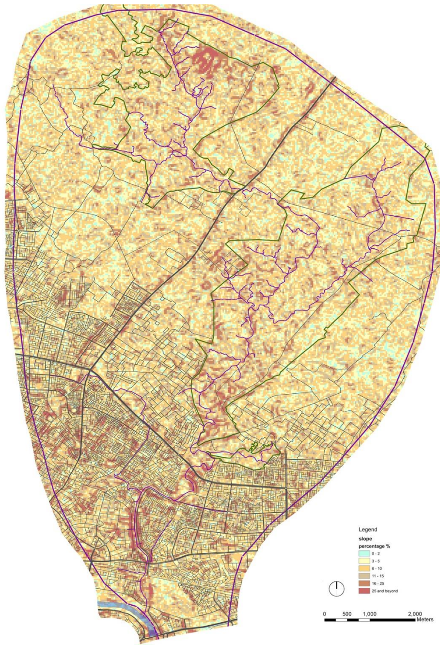
Figure 3-3 Slope map of the Kukrail basin (based on USGS database, Arcmap GIS)
