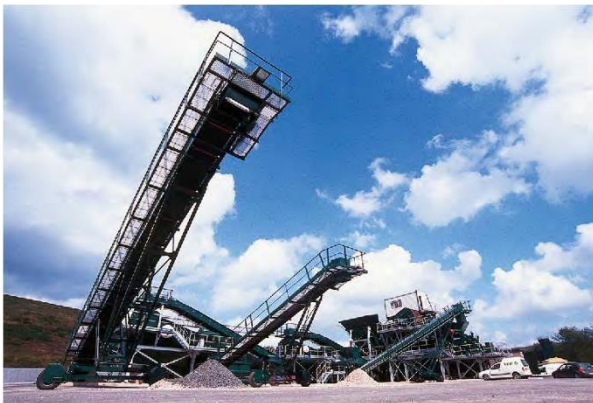
Rubble waste • Processing: sortinging and en breaking • Production: granulate and granulate products
