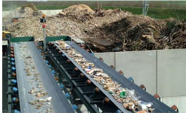
Wood waste • Processing: sorting and reducing • Production: raw material (chipboard industry) fuel (stoke in power station)
