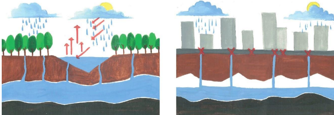
Figure 53: Sketch showing the major reason for ground water depletion
