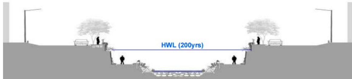
Figure 25: Section of estimated flood level 200 yrs
